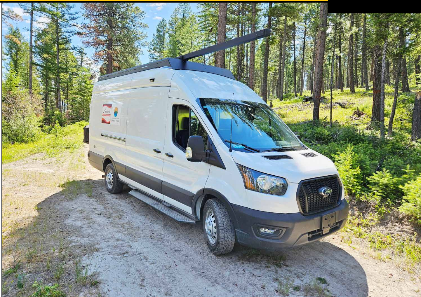
The SMART FIRES mobile lab can be used to sample smoke off-grid, while parked or driving, and can power over 5 kW of science equipment. Image courtesy of Wade Permar.
