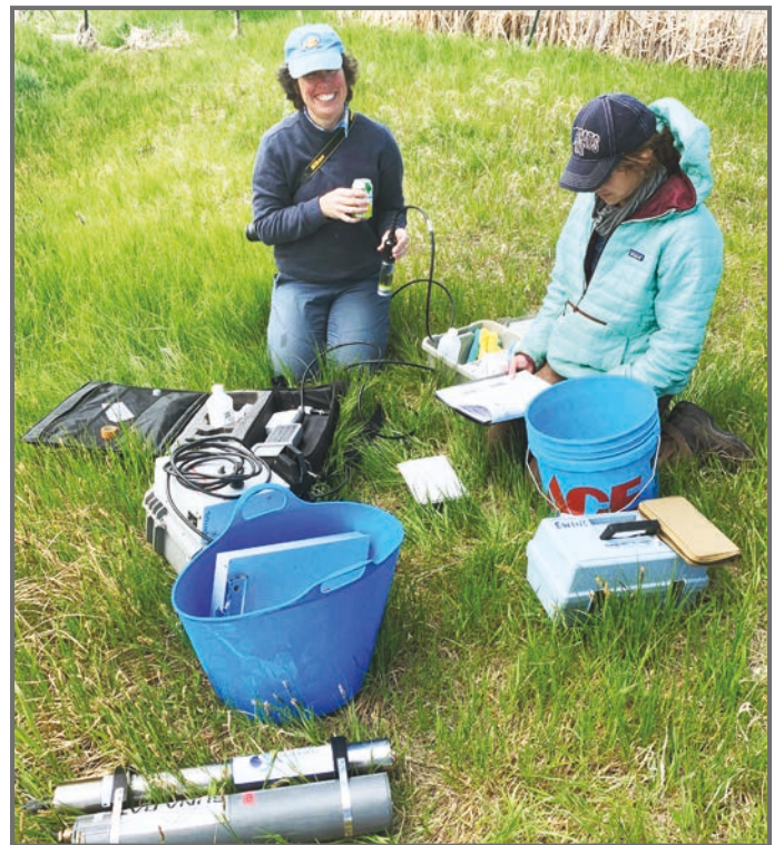
Stephanie Ewing and PhD student Caitlin Mitchell calibrate a multimeter in preparation for sampling a JRW creek. A SUNA sensor in the foreground awaits deployment. The sample will serve to verify the sensor measurement and provide ancillary data. Photo credit: Ray Callaway
