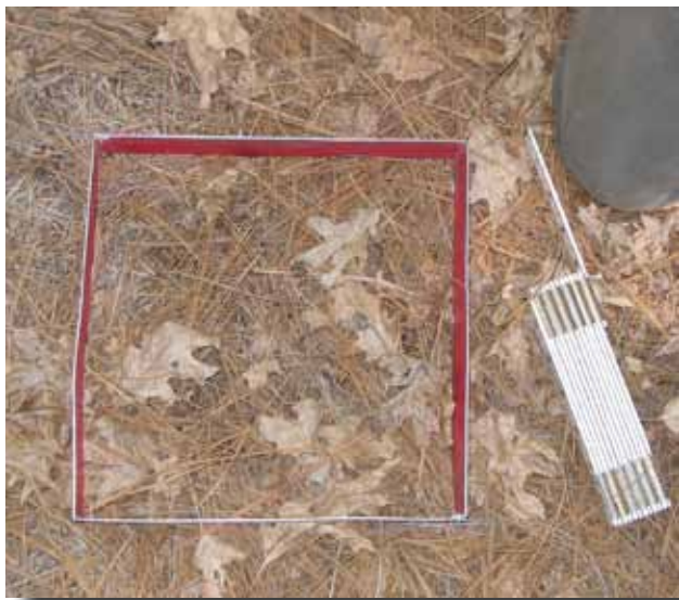
Figure 12—Preparing to collect litter and duff samples.
