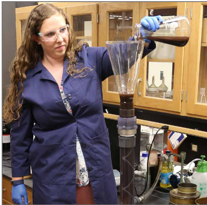
Teagan Leitzke, who was a CREWS graduate student at Montana Tech, pours a slurry of magnetite and water into the continuous flow metal recovery system. The slurry flows through the static mixer column to a magnet, where the magnetite is collected, and water continues to flow out of the system. Photo credit: Amanda Badovinac.
